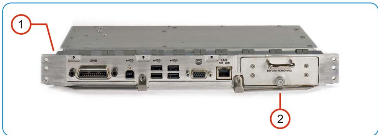
Figure 8-2 Processor Assembly with Removable Disk Drive
